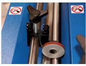
The positioning of the perforator overcomes any potential issues caused by poor film roll profiles and allows greater speed and decurl angles minimising web breakage.
