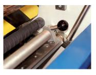
A decurl bar, which may be altered on the run, is fitted to assist in giving a flat result.
