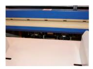
The electronically adjustable burster automatically separates sheets up to B3 size whilst fans provide a cushion of air to support the sheet as it is delivered into the catch tray.
